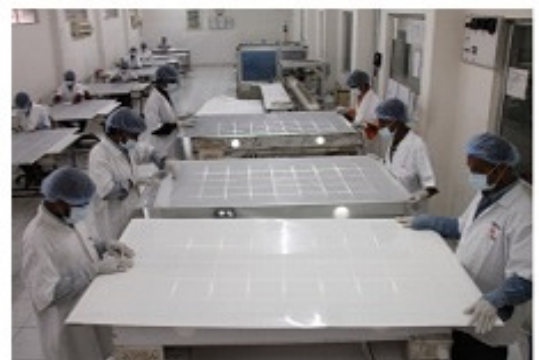
Tabbing, Stringing & Lay up operations: Photon Solar PV module line
